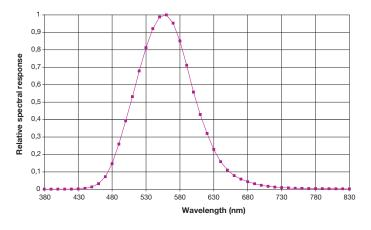
Figure 2. HD2021T6 probe relative spectral response
