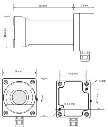
The probe uses a silicon photodiode and a set of filters to correct the spectral response curve to make it equal to that of the human eye (photopic response). Figure 2 shows the trend of the relative spectral response according to the wavelength.
