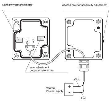
Figure 5. Connection diagram for HD2021T... with current output
